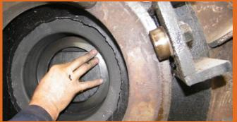
PIC FIVE BELOW LEFT: This one shows that the upper refractory plate in situ into the outer nozzle and the graphite ring surrounds the plate to ensure that the joint is protected from plate leaks.
