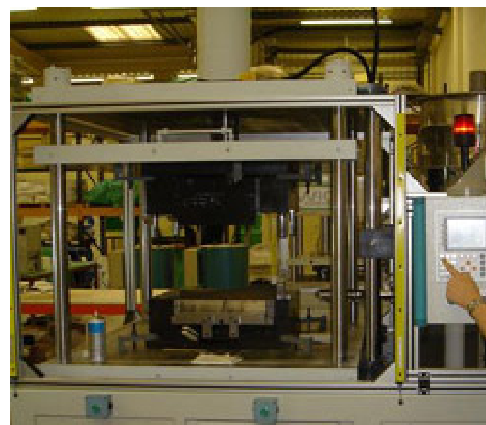
Pictured above, one of CIC's injection presses, designed to accommodate transfer core tooling
