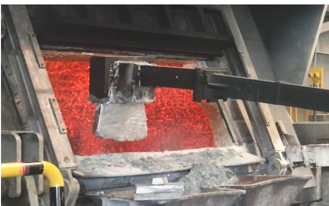
Amourcast high fracture toughness composite shapes for skimmers and stirring booms, door surrounds and nose ring blocks
